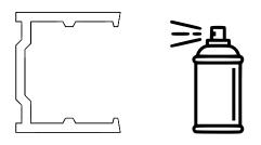
3. Apply silicone adhesive to the inside bottom of the channel. Then, insert the Trace fixture (starting from the power side) into the channel and carefully press along the length of the fixture. The connectors and end caps do not fit into the channel and will overhang on the outside ends.
