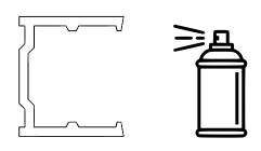
3. Apply silicone adhesive to the inside bottom of each mounting clip and insert the Trace fixture (starting from the power side) into each mounting clip carefully until the fixture is fully secure.
